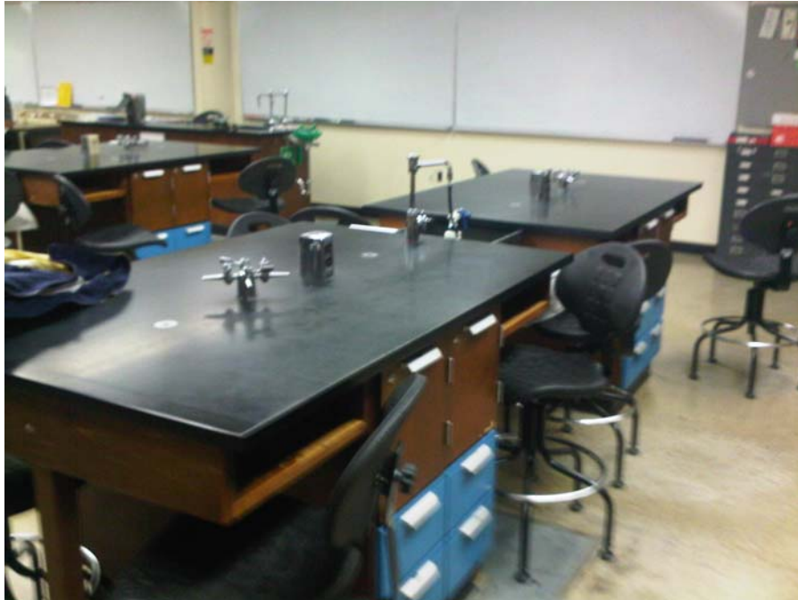
Lab table with "center sink, gas, water and electric", typical for biology labs
